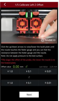
3. After adjusting the distance between the nozzle and the build plate, follow the prompt on the screen to load Hyper Speed PLA filament.
